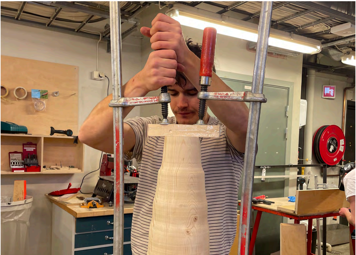
Vertical glulams The other glulam vase was glued with the wooden fibers in the vertical direction
