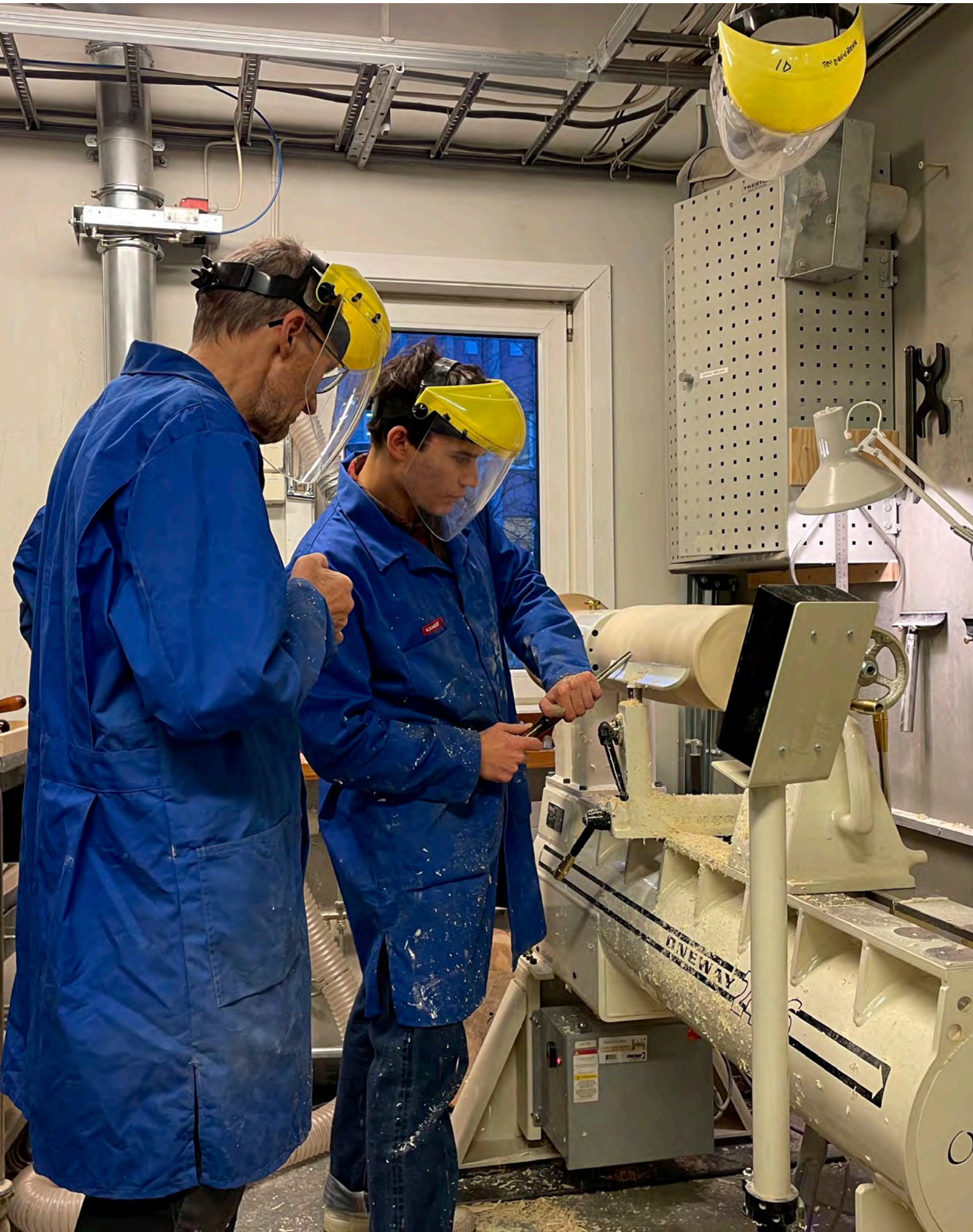
Turning Both vases were turned on the lathe. The one with vertical fiber direction was easier to work with.
